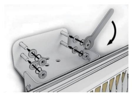
1.6. Finally, if necessary, you have the option of adjusting the angle of the heating head to your individual needs by loosening the two locking screws.
