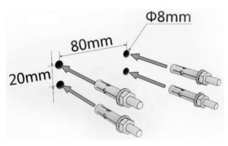
1.4. Take the dowels supplied and fix them in the drilled holes. Then loosen the nuts, washers and spring washers from the dowels.
